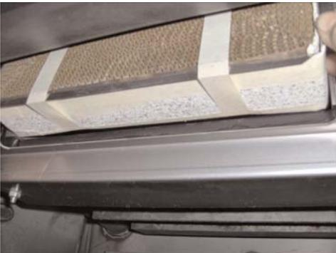
Since the combustor is only 2" deep, there is ample room to lift the new combustor into place. **REMEMBER TO HAVE THE TAB ACROSS THE BOTTOM EDGE OF THE COMBUSTOR AS IT IS INSTALLED.** Slowly push the combustor in at the top, apply even pressure to the left and right corner. This will allow for better view of the bottom edge for the final fitting. **DO NOT FORCE THE COMBUSTOR INTO THE DOME. TAKE YOUR TIME AND WORK IT INTO PLACE SLOWLY.**
