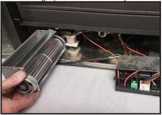
5. Slide the blower along the back wall until it reaches the stop flange, then feed the blower wires underneath the gas supply to the front as shown.
