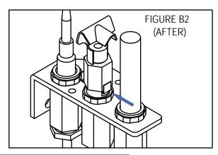
3) RE-TIGHTEN THE PILOT TARGET HEX FITTING UNTIL THE PILOT TARGET ALIGNS WITH THE THERMOCOUPLE & THERMOPILE AS SHOWN IN FIGURE C. USE CAUTION TO AVOID BENDING ORIFICE STRIP BY IMPROPER PLACEMENT OF END WRENCH.
