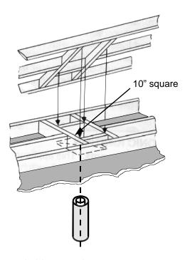
Use a suitable round or square support through the roof. Ensure adequate heat shield protection is provide. See diagram and chart for minimum protection.
