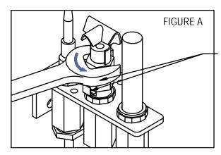
AVOID CONTACTING ORIFICE STRIP WITH END WRENCH. FAILURE TO DO THIS CAN CAUSE DISTORTION OF THE ORIFICE STRIP WHEN LOOSENING OR TIGHTENING.
