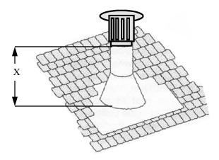
To prevent water seepage install the flashing with upper portion slid under the roofing material and the lower portion over the roofing material.
