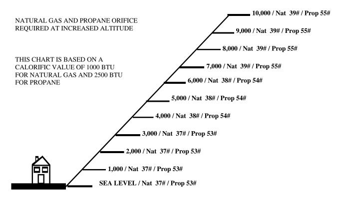
Check with your local gas supplier for correct calorific value (btu rating).
