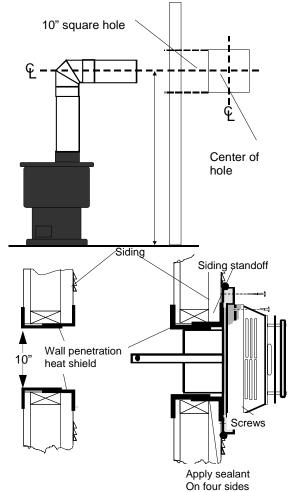
Before sliding the pipe into the termination ensure that you slide the decorative wall thimble cover and penetration heat shield over the pipe.
