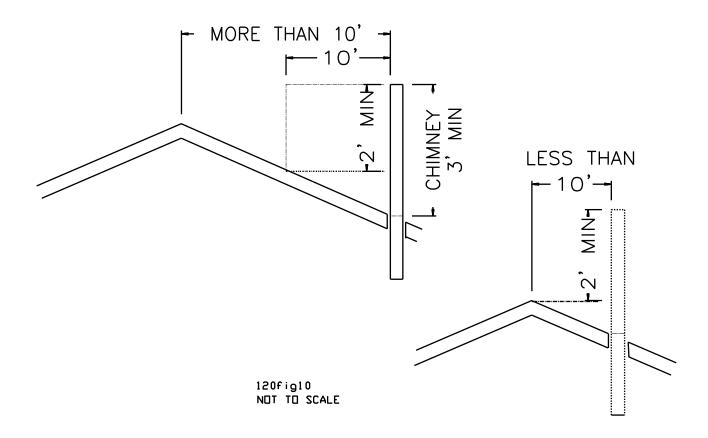
The height requirement is necessary in the interest of safety and does not necessarily assure proper flue draft. Use a minimum total system height of 12 feet, measured from the stove flue collar to the top of the chimney, not including the chimney cap.
