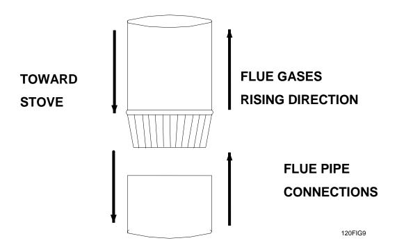
Recommended draft is .03 in. water COLUMN. It is unsafe to operate the furnace with more than .06 in. water column draft, use a barometric control, if necessary, to achieve this.
