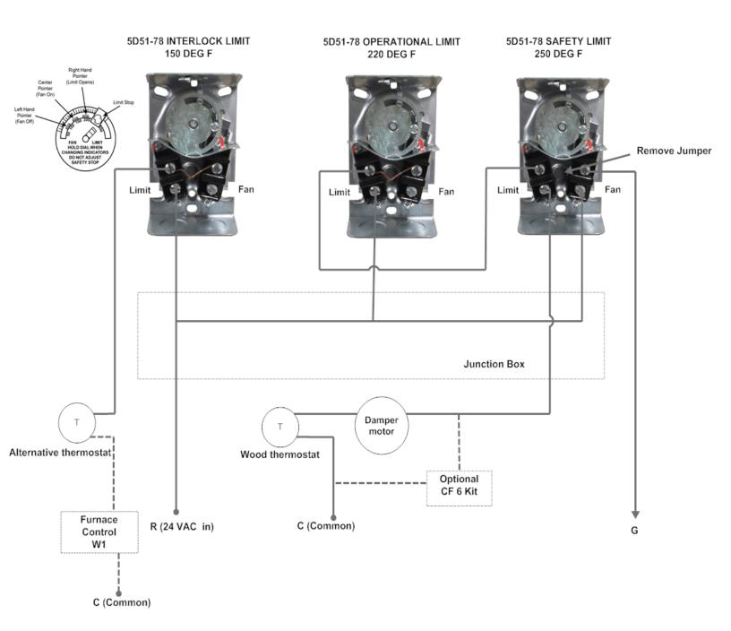
You must connect the alternate furnace thermostat through the interlock limit switch to provide interlock lockout of the alternate furnace when the wood plenum rises above 150 degrees.
