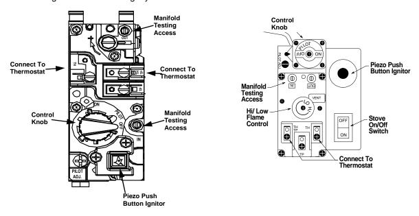
NOTE: The knob cannot be turned from PILOT to OFF unless the knob is pushed in slightly. DO NOT FORCE.
