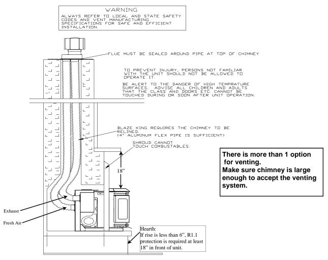
THE BLAZE KING INSERT CAN ONLY BE INSTALLED IN A MASONRY FIREPLACE OR A LISTED WOOD BURNING "O" CLEARANCE FIREPLACE MODELS.
