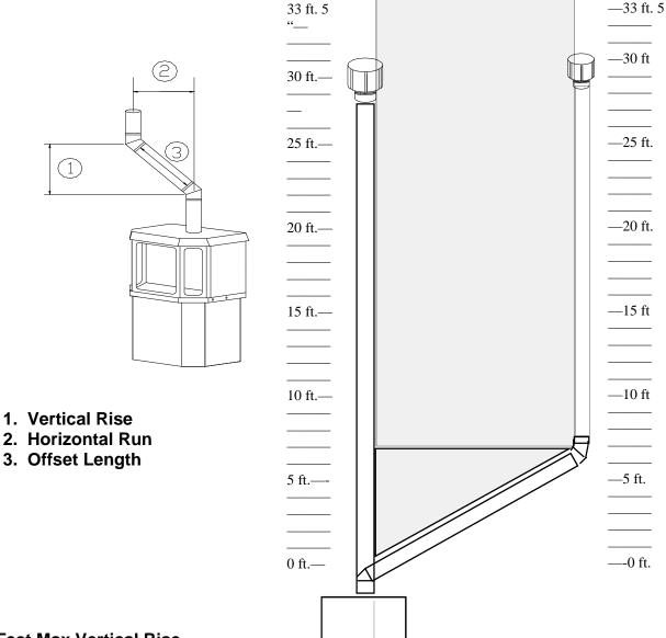
31 Feet Max Vertical Rise 6 Feet Max Horizontal Offset 9' Min. Vertical Rise
