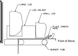
**EMBER PLACEMENT:** Place embers directly on the front burner tube, leaving a 1/4" gap between the front log and the embers.
