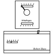
NOTE: If using any one of the thermostat controls, the manual switch must be in the OFF position. If it is left ON the stove will continue to run and the thermostats will have NO control over the stove.
