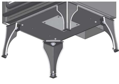
4. Utilizing the key holes on the top of the case, slide the case into place by pushing it against the bottom of the stove and then pushing it towards the back of the stove (use the half turned in bolts as guide pins).
