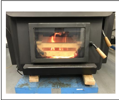
Run 1 – Newly Loaded Stove
