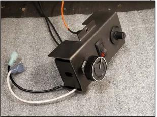
12. Connect the black "W" wire from the rheostat to the white "W" wire from the power cord.
