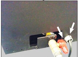
8. Remove the two screws holding the control panel and dissconnect the switch wires from the valve...
