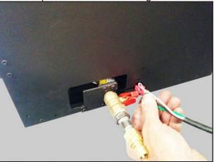
6. Slide the loomex bushing into the case hole.
