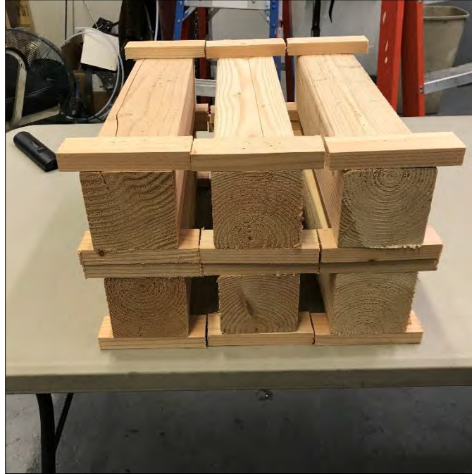
Typical Test Fuel Load Configuration
