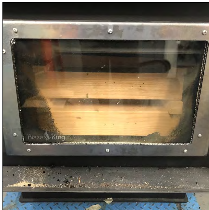
Typical Test Fuel Loaded in Test Stove
