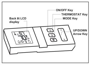
Fig. 19: Remote LCD Display
