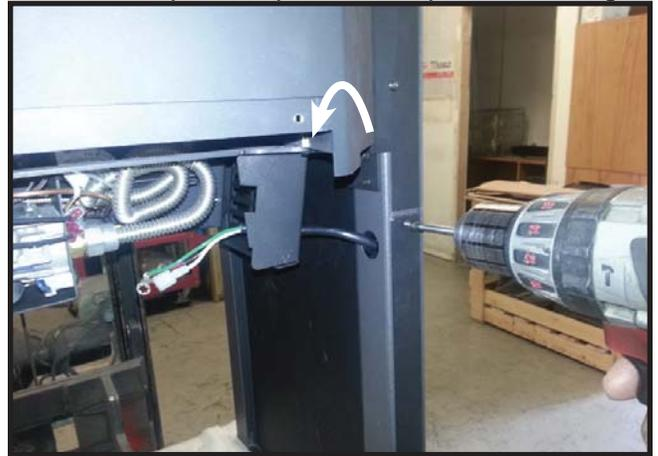
2. Feed power cord assembly wires through slot and plastic bushing of leg.
