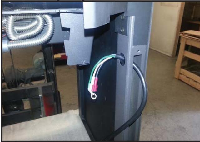
5. Screw the bottom of the power cord plate to the leg.
