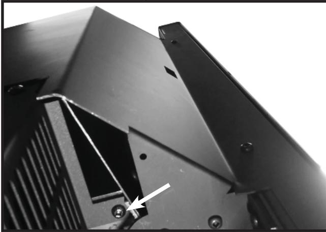
4 screws to secure the back.
