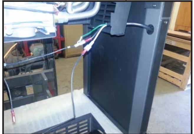
9. Slide the snap disk into the snap disk bracket that is above the rheostat on the firebox bottom. Ensure the snap disk tabs are both seated into the bracket.
