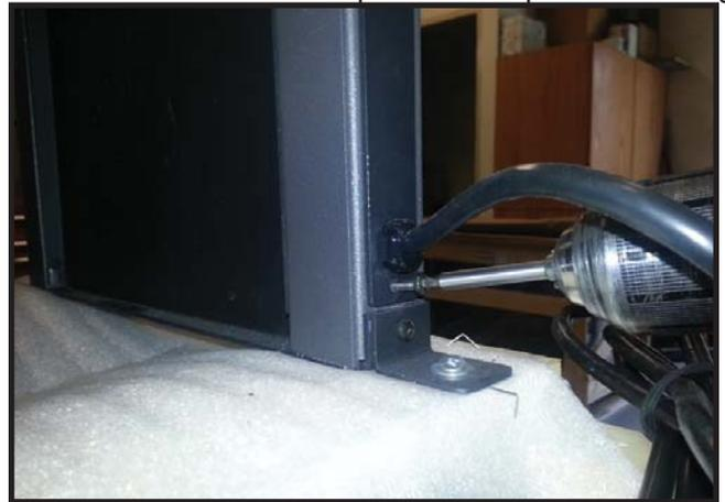
3. Feed power cord assembly wires through the control housing's plastic bushing.
