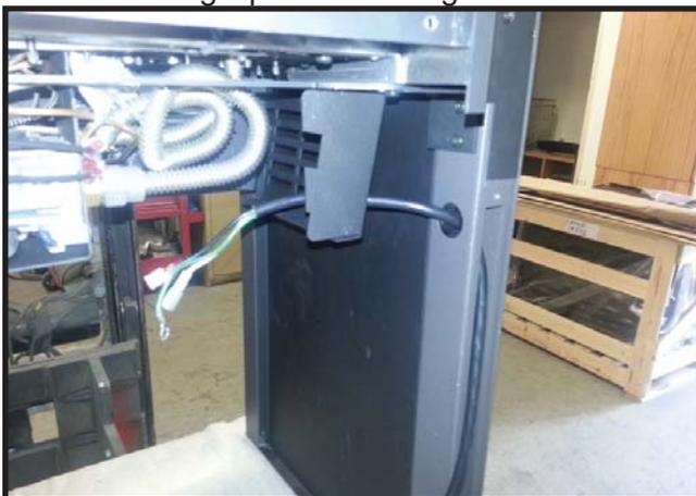
6. Lay blower assembly on blower box between legs. Slide the fan rheostat into the control plate hole as shown.
