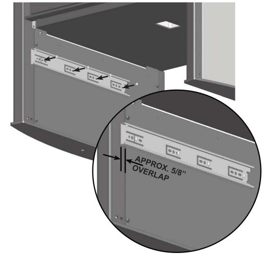
3. Attach drawer slides to side panels with the included screws. Use the holes shown below.
