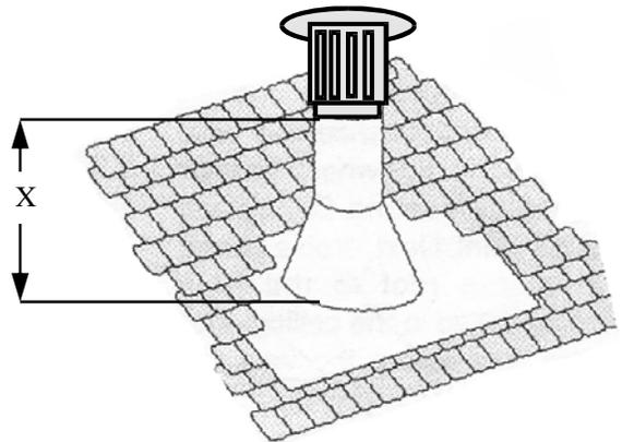
To prevent water seepage install the flashing with upper portion slid under the roofing material and the lower portion over the roofing material.
