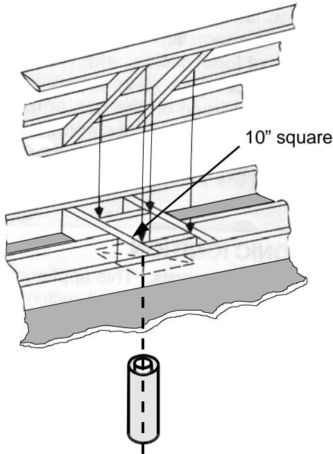
Use a suitable round or square support through the roof. Ensure adequate heat shield protection is provide. See diagram and chart for minimum protection.
