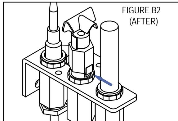
3) RE-TIGHTEN THE PILOT TARGET HEX FITTING UNTIL THE PILOT TARGET ALIGNS WITH THE THERMOCOUPLE & THERMOPILE AS SHOWN IN FIGURE C. USE CAUTION TO AVOID BENDING ORIFICE STRIP BY IMPROPER PLACEMENT OF END WRENCH.
