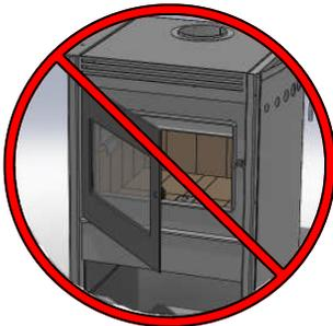
**Never** burn the stove with the loading door open. Never block free airflow through vents on this appliance.
