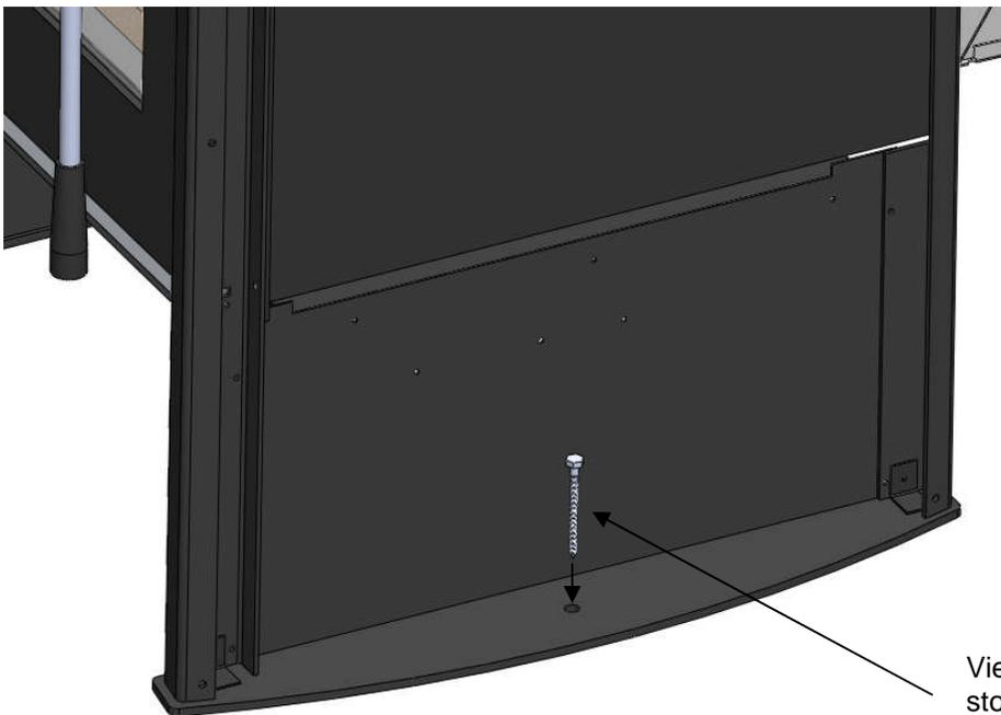
**In mobile home installations, the stove must be securely fastened to the floor using the tie-downs provided in the Outside Air kit.** (To access the screw down hole, remove side shields (see page 23)).
