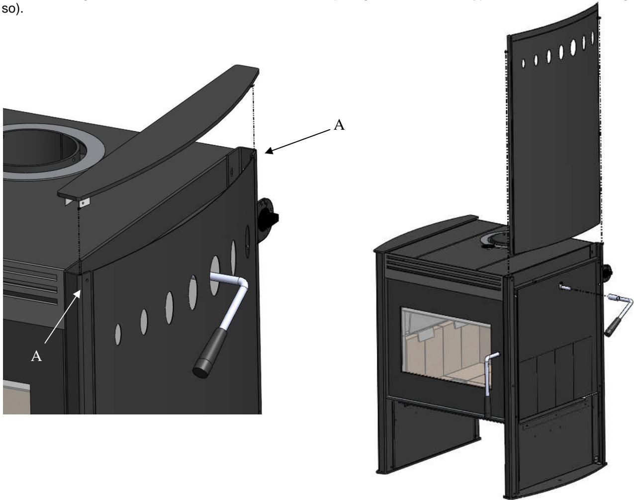
If you like to install the flat versus the curved shields or vice versa, the matching cover plate on the bottom need to be replaced too. This can be done by undoing the two screws (B) holding the bottom plate in place. An extra person or jack might be required to lift the one side of the stove. Check stove pipe and possible fresh air connection before doing so. If installed in mobile home, remove floor anchor prior to lifting stove.
