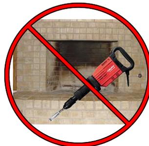
Do not make any changes or modifications to an existing masonry fireplace or chimney to install this appliance. Do not make any changes to the appliance to increase combustion air.
