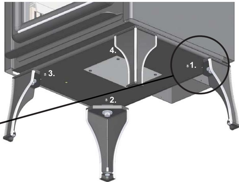
4. Utilizing the key holes on the top of the case, slide the case into place by pushing it against the bottom of the stove and then pushing it towards the back of the stove (use the half turned in screws as guide pins).
