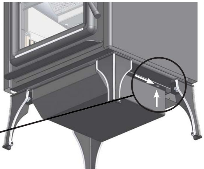
5. Once the case is in position, finish tightening the four bolts into the stove bottom.
