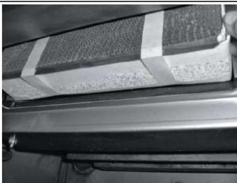
6. Since the combuster is only 2" deep, there is ample room to lift the new combuster into place. **REMEMBER TO HAVE THE TAB ACROSS THE BOTTOM EDGE OF THE COMBUSTOR AS IT IS INSTALLED.** Slowly push the combuster in at the top apply even pressure to the left and right corners. This will allow for a better view of the bottom edge for the final fitting. **DO NOT FORCE THE COMBUSTOR INTO THE DOME. TAKE YOUR TIME AND WORK IT INTO PLACE SLOWLY.**
