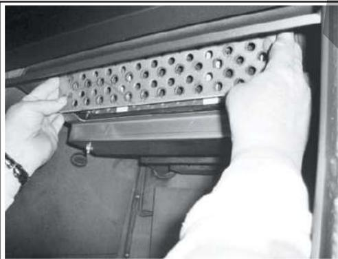
2. Once you remove the flame shield, you'll find the combustor. The honeycomb combustor can be made of different materials such as cordierite, mulite or even stainless steel. They are all the same with regard to removal and caution should be taken so as to not drop or damage the combustor. If your combustor has never been cleaned according the manufacturers directions, you may wish to clean the combustor before replacing it with a new combustor, see "CATALYTIC COMBUSTOR CLEANING" on page 28.
