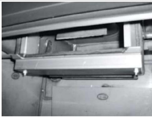
4. Using the same screwdriver or pocket knife, scrape any old gasket from the surface areas of the dome. The dome is the housing that surrounds the combuster. If you clean your existing combuster, you'll need to order replacement combuster gasket. It is always a good idea to have a spare combuster gasket on hand prior to performing any maintenance. If you purchase a new combuster a new gasket will already be applied to the combuster.
