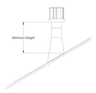
Install the flashing with upper portion slid under the roofing material and the lower portion over the roofing material.
