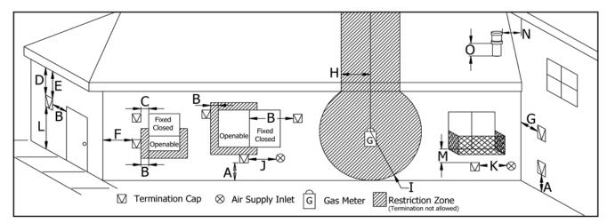
Fig.13 VENT TERMINATION RESTRICTIONS, REFER TO Table 1
