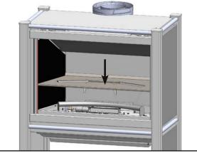
10. Place the floor glass on top of the floor plate assembly. (Fig.14) NOTE: SMOOTH SIDE SHOULD FACE UP.
