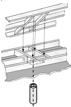
Use a suitable round or square support through the roof. Ensure adequate heat shield protection is provided.
