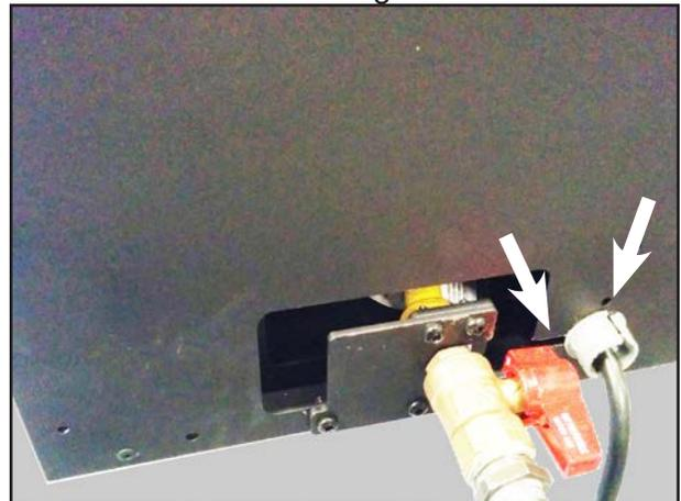
8. Remove the two screws holding the control panel and disconnect the switch wires from the valve..
