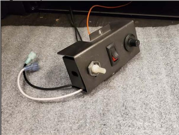
11. Attach star washer, nut, and knob to rheostat post.
