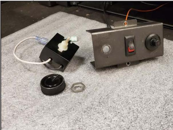
10. Affix the rheostat to control panel, note the alignment pin location.
