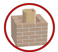
This appliance must be connected to a listed high temperature (**UL1777,ULC635,ULC640**) approved masonry chimney with a flue liner.
