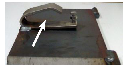
APPLY LUBE TO THE UNDER SIDE OF THE BYPASS RAMP
