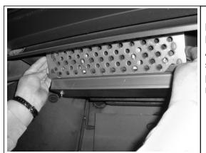
1. The appliance must be cool to touch, having gone at least 12 hours without being burned. A combustor can reach 1400F and hold temperatures for several hours, even after the fire is out. After waiting 12 hours, begin by removing the flame shield by simply lifting the shield off the two tabs at either lower corner. Pay particular attention to orientation of the flame shield in order to reinstall in the correct position.
