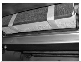
6. Before installing, align the combustor within the opening of the dome housing. Slowly push the combustor in at the top and apply even pressure to the left and right corners. This will allow for a better view of the bottom edge for the final fitting. **DO NOT FORCE THE COMBUSTOR INTO THE OPENING. TAKE YOUR TIME AND WORK IT INTO PLACE SLOWLY.**
