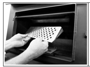
7. Once the combustor is fully reinserted into the opening of the dome housing, replace the flame shield. Note the flame shield sides are shaped like a triangle. The point of the triangle should face down to install correctly. Do not operate your appliance without the flame shield in place. The flame shield protects the face of the combustor against direct flame impingment and potential collisions when loading fuel.
