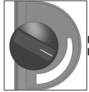
ROTATE COUNTER CLOCKWISE FOR REDUCED HEAT OUTPUT
