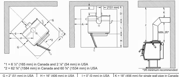
Ember protection shield (not required to have an insulation value) is to be listed under UL 1618-2009 (type 1) and must have a minimum size of:
