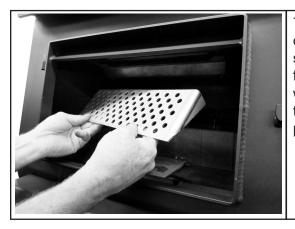
7. Once the combustor is fully reinserted into the opening of the dome housing, replace the flame shield. Note the flame shield sides are shaped like a triangle. The point of the triangle should face down to install correctly. Do not operate your appliance without the flame shield in place. The flame shield protects the face of the combustor against direct flame impingment and potential collisions when loading fuel.
