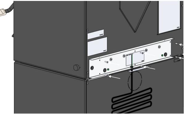
4. With the fan kit body in place, install the outer cage by fastening x2 sheet metal screws from the top side. Finish off the install by press fitting the rheostat knob onto the protruding arm.
