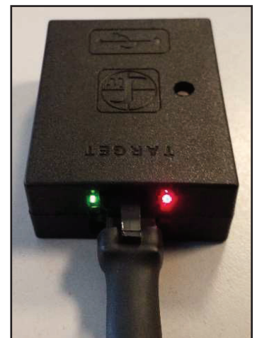
Fig. 3: WIFI DONGLE CONNECTED TO THE IFC
