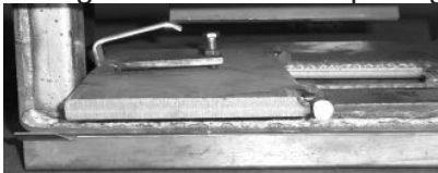
BYPASS DOOR REMOVAL THROUGH COMBUSTOR OPENING
