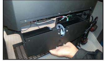
5. Secure the fan by fastening x6 screws to the appliance (note: x2 screws fasten into the firebox bottom).
