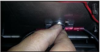
Install the lower wire cover by using x4 screws to fasten it to the underside of both the right and left control panel sides.
