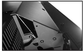
4. Position the rheostat housing into the hole on the rear side of the control housing panel.
