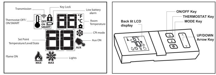
Fig. 19: Remote LCD Display
