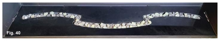
There is a precise amount of burner ember media is provided to cover up the burners in the open area of the floor glass. Distribute the embers evenly on either side of the ember shield until all the burners are covered. (Fig. 39 & 39a)
