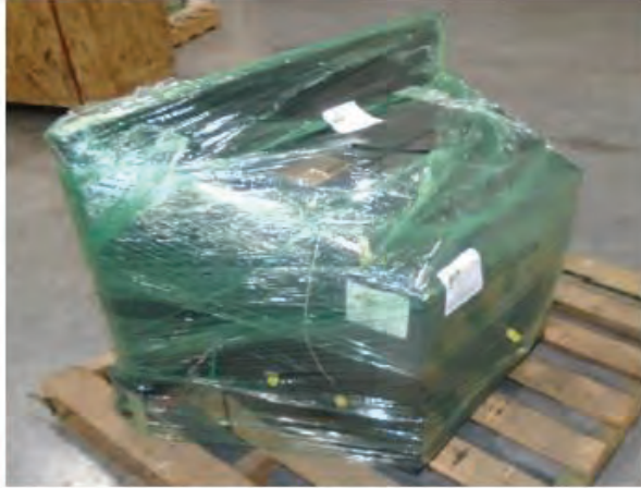
Appliance Shrink-Wrapped and three additional seals added
