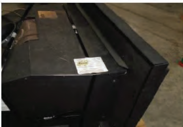
Appliance banded to pallet, then two seals applied over banding
