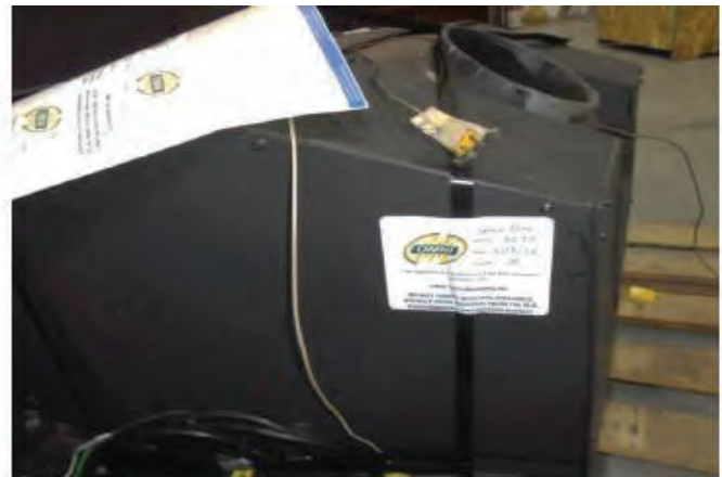
Appliance banded to pallet, then two seals applied over banding
