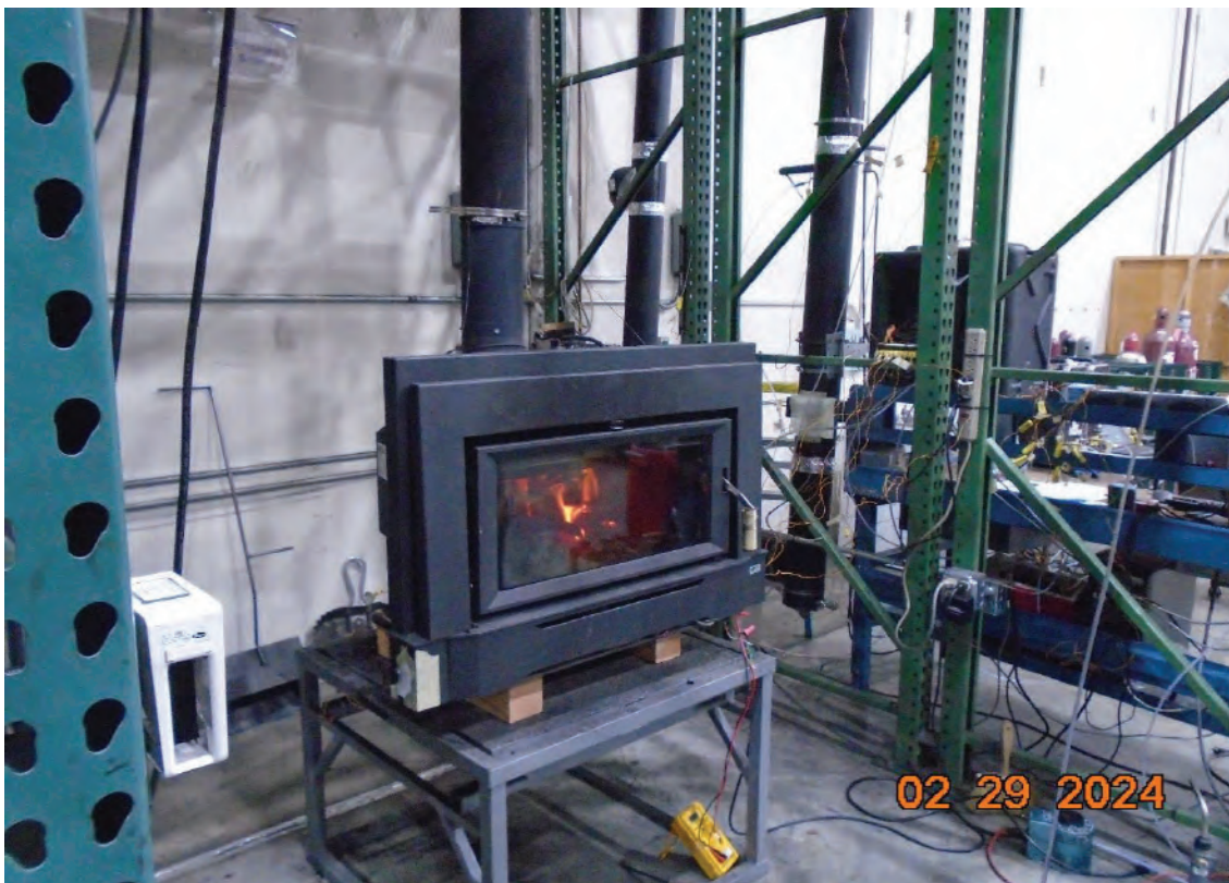
Figure 10 - Close-up of Appliance installed in test booth
