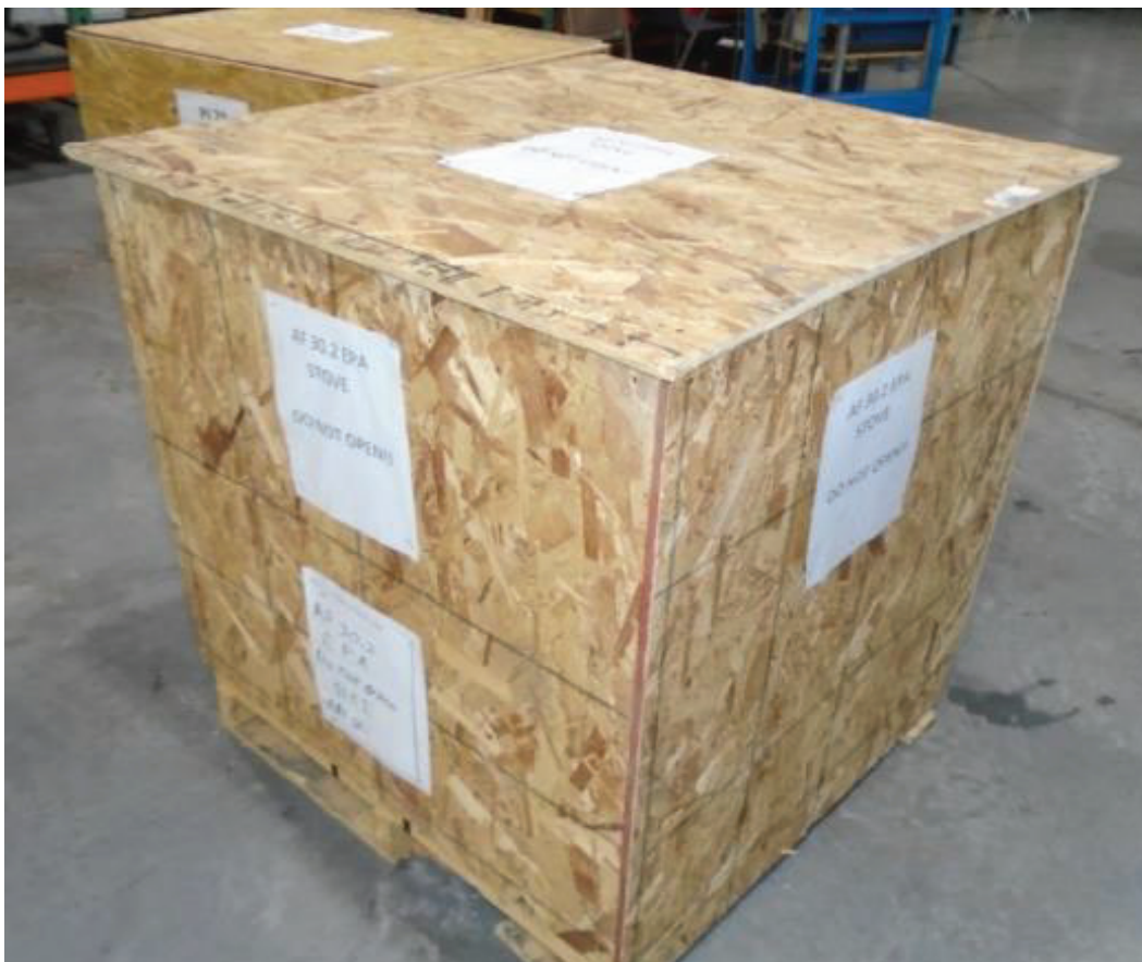
Crating placed over sealed test specimen
