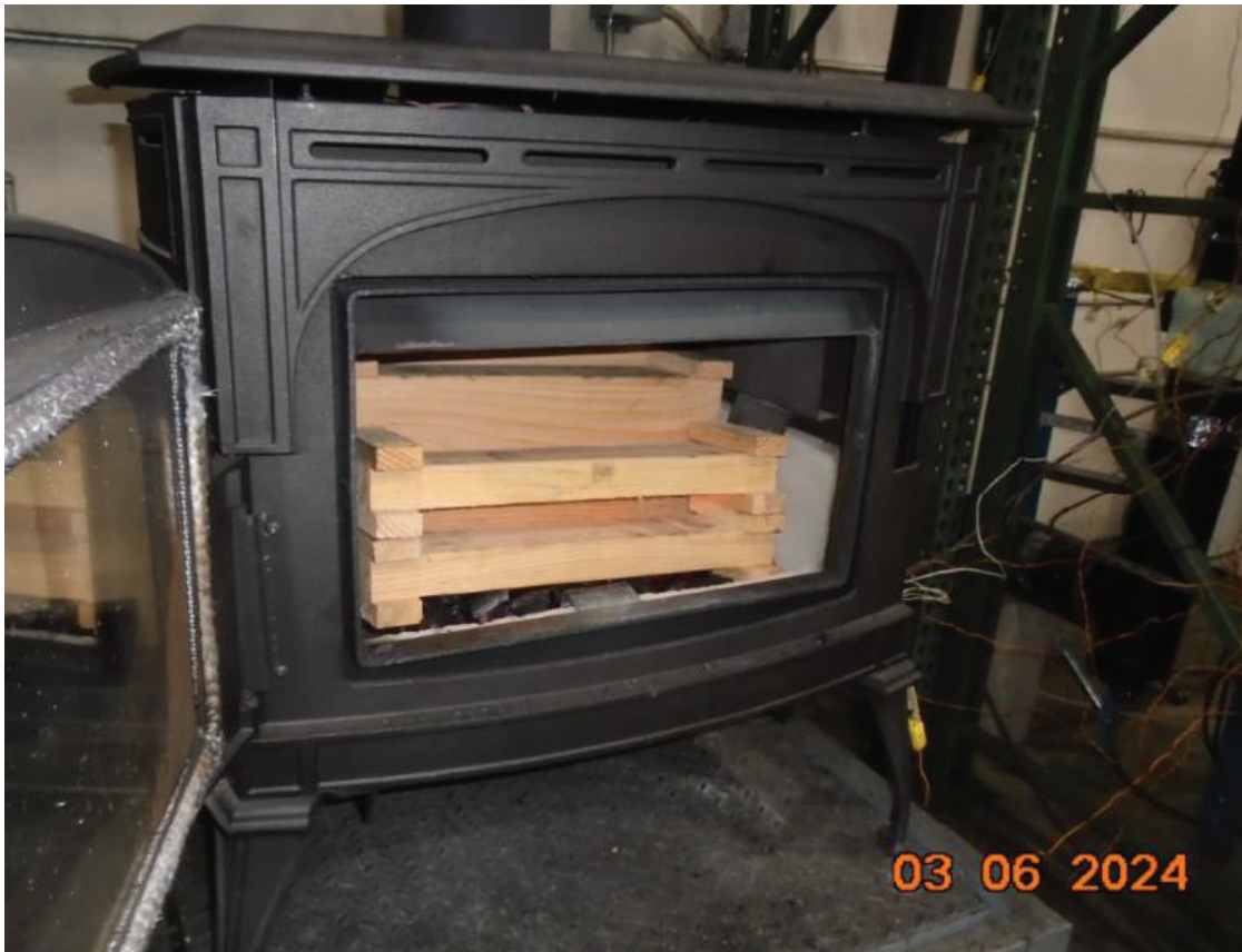
Figure 29 - Run 4 - Loaded Stove
