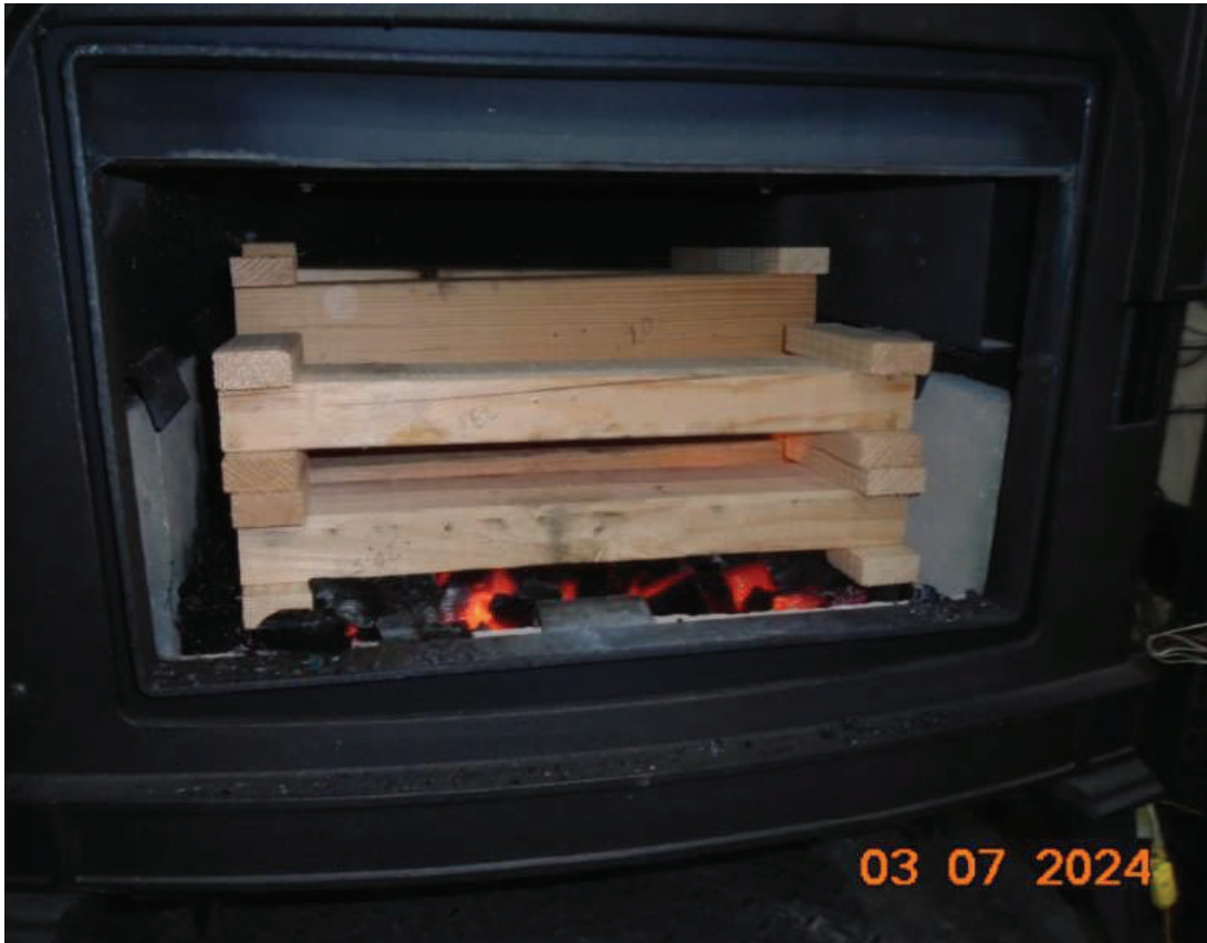
Figure 33 - Run 6 - Loaded Stove
