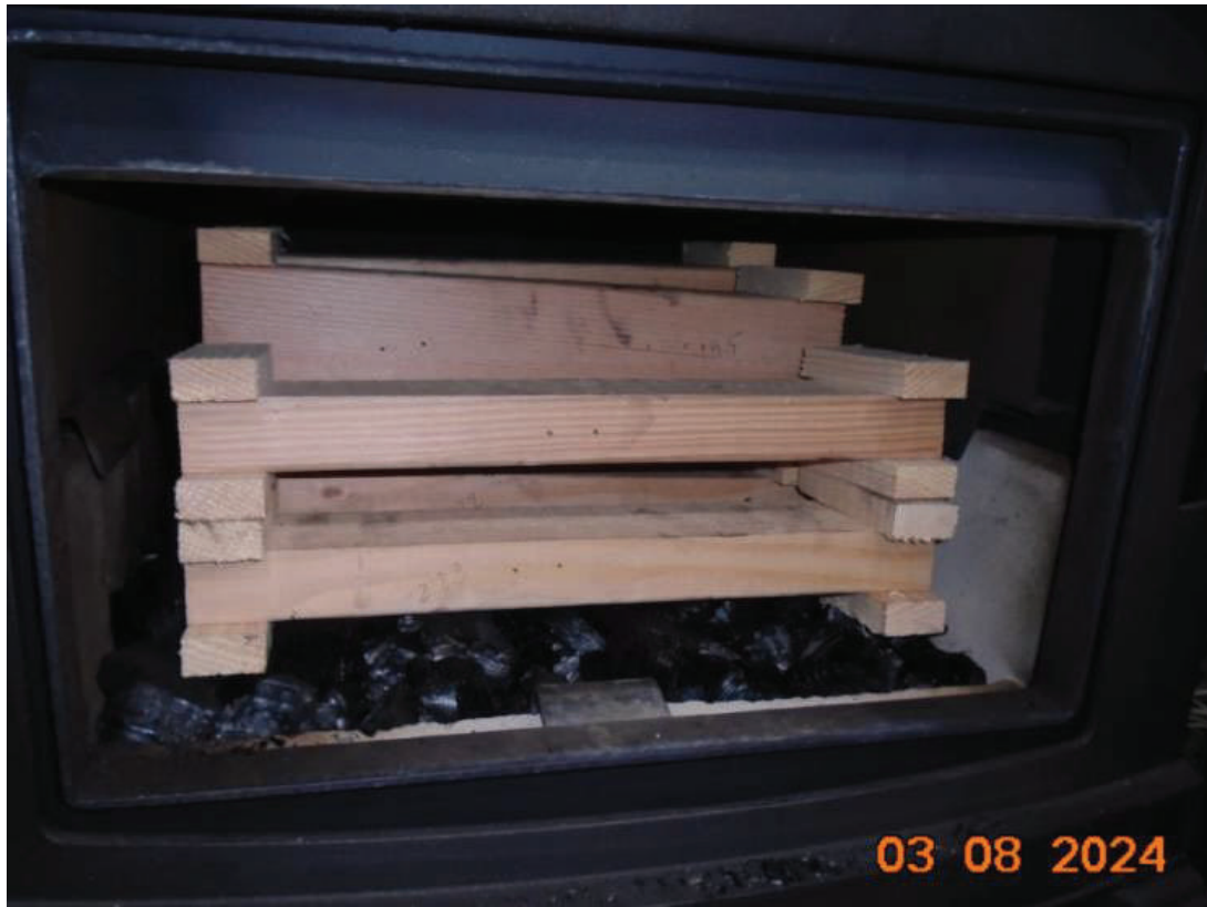
Figure 35 - Run 7 - Loaded Stove
