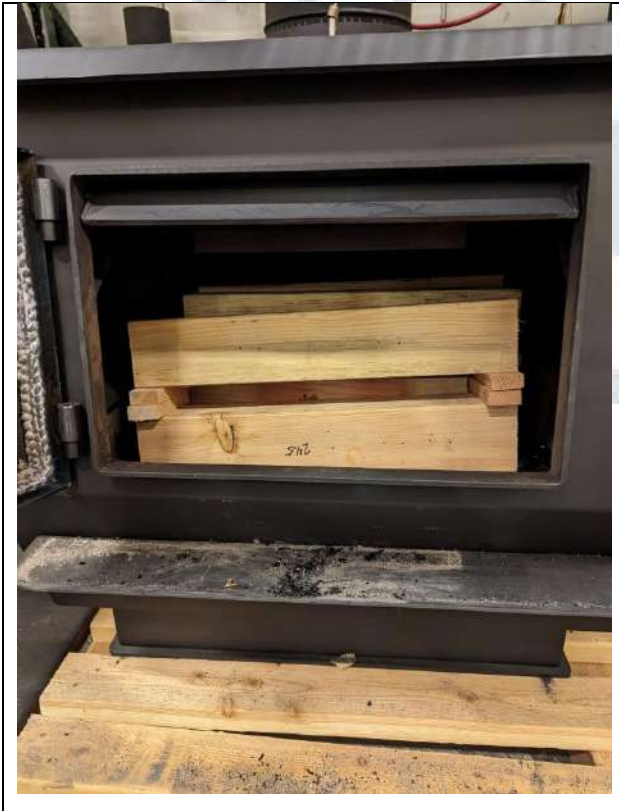
Test Fuel Loaded in Stove
