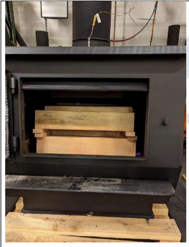
Test Fuel Loaded in Stove
