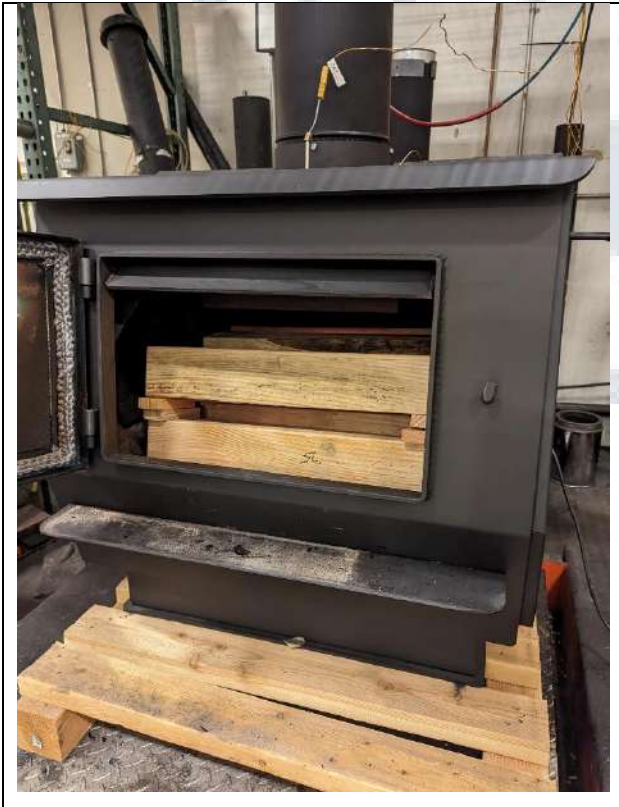
Test Fuel Loaded in Stove
