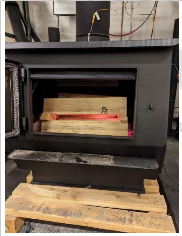
Test Fuel Loaded in Stove
