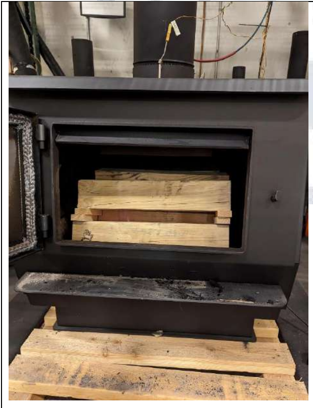
Test Fuel Loaded in Stove
