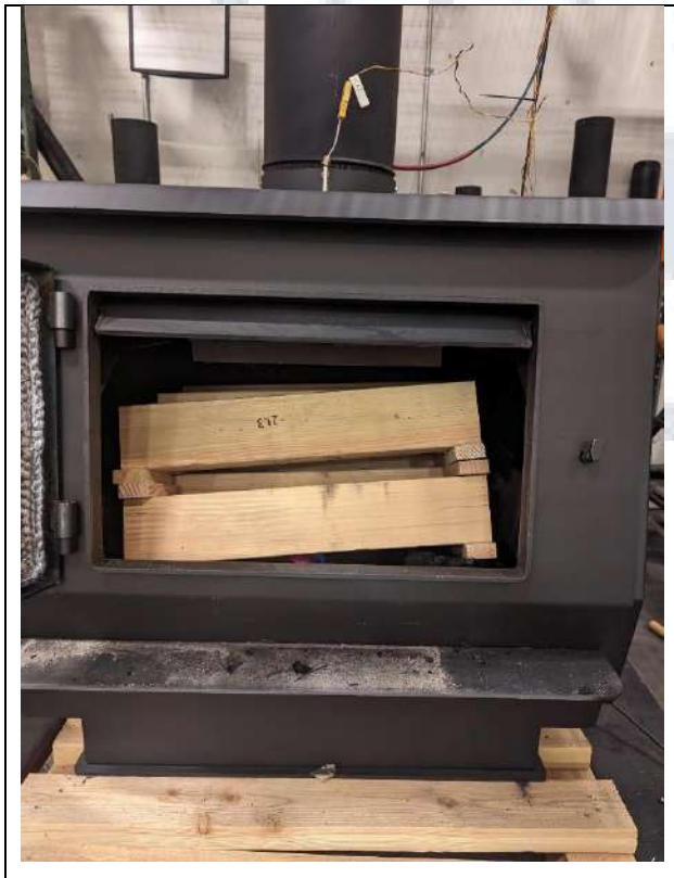
Test Fuel Loaded in Stove
