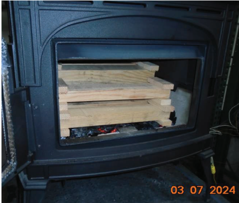
Figure 32 - Run 5 - Freshly Loaded Stove
