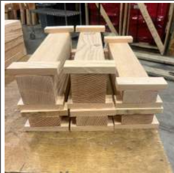
Test Fuel Front/Side View
