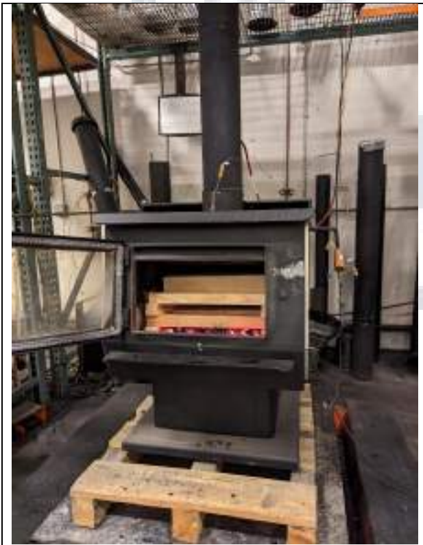
Test Fuel Loaded in Stove
