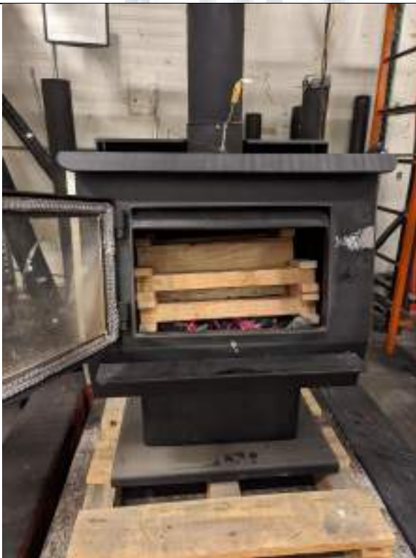
Test Fuel Loaded in Stove
