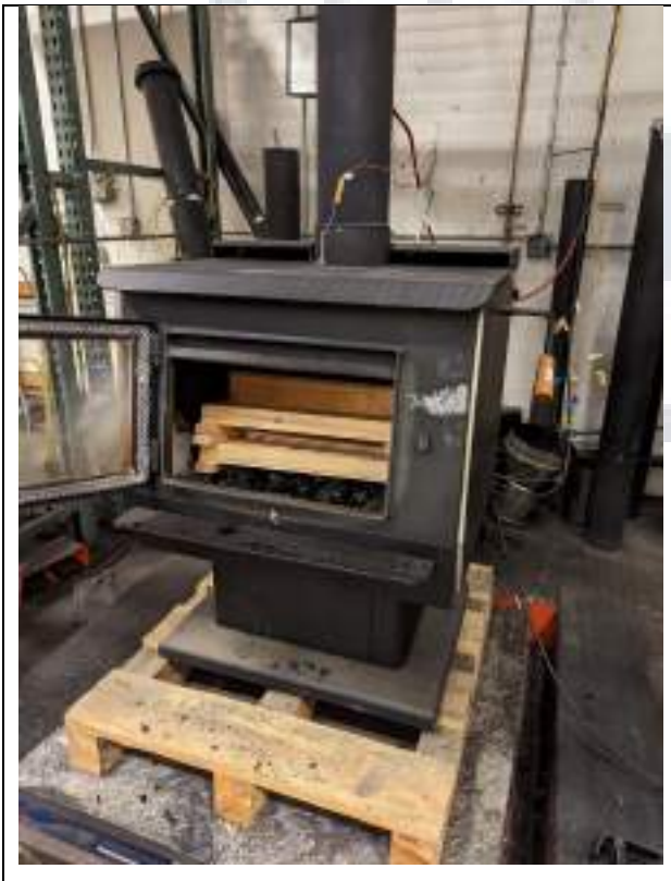
Test Fuel Loaded in Stove
