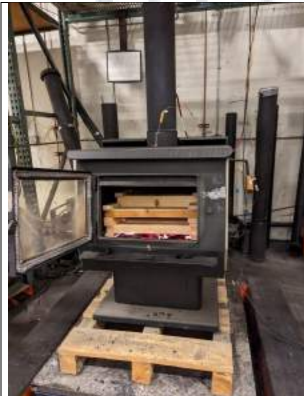
Test Fuel Loaded in Stove
