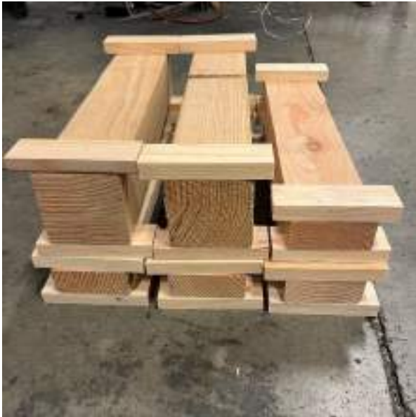
Test Fuel Front/Side View
