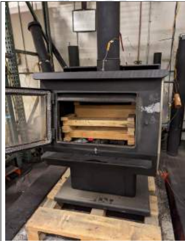
Test Fuel Loaded in Stove
