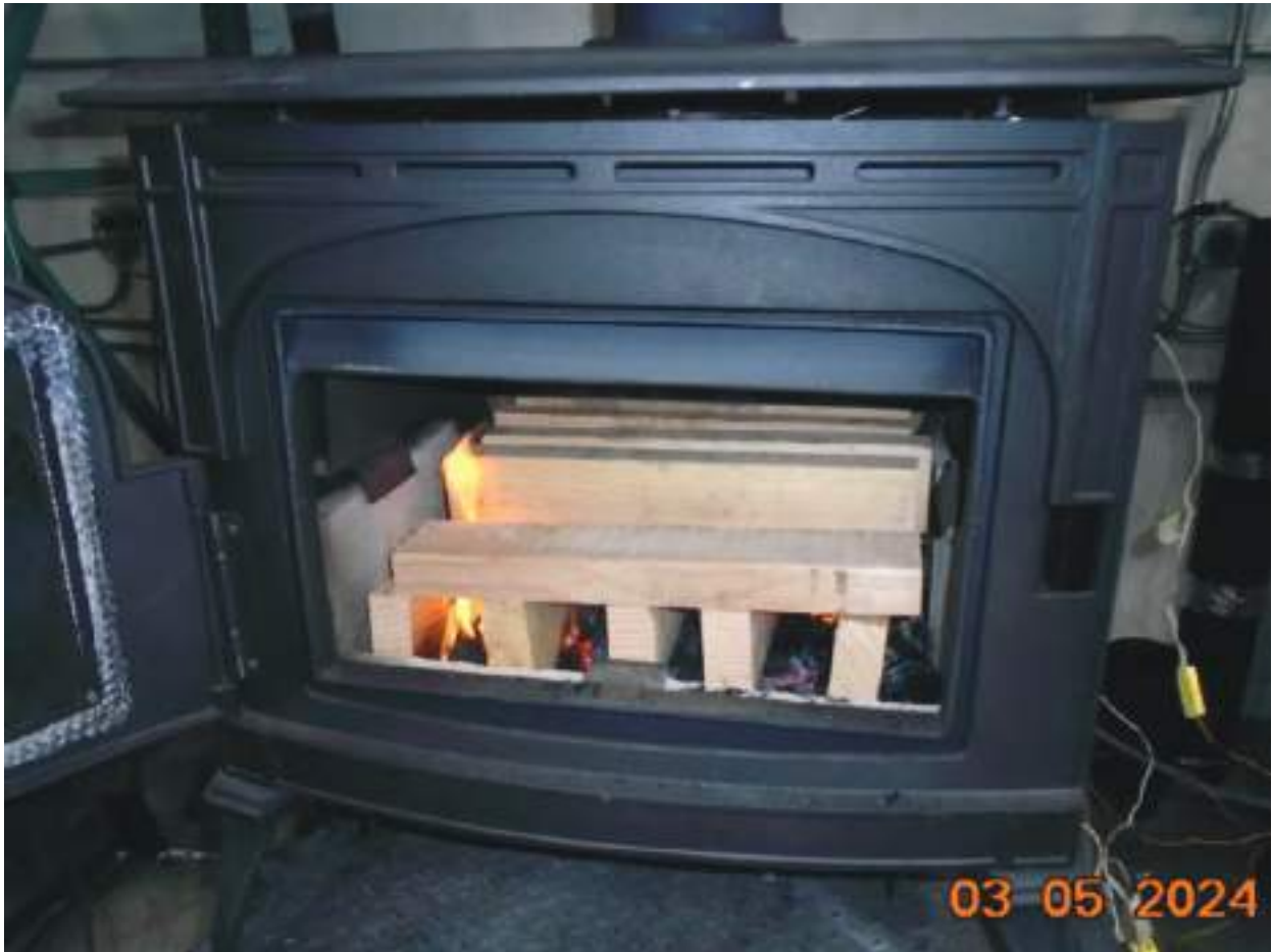
Figure 24 - Run 1 - Freshly Loaded Stove
