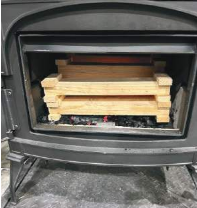
Figure 26 - Run 2 - Freshly Loaded Stove
