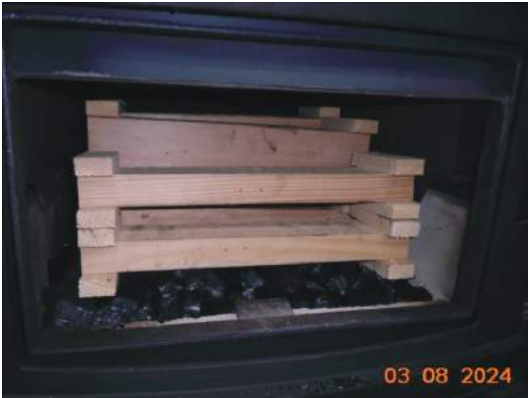
Figure 36 - Run 7 - Loaded Stove
