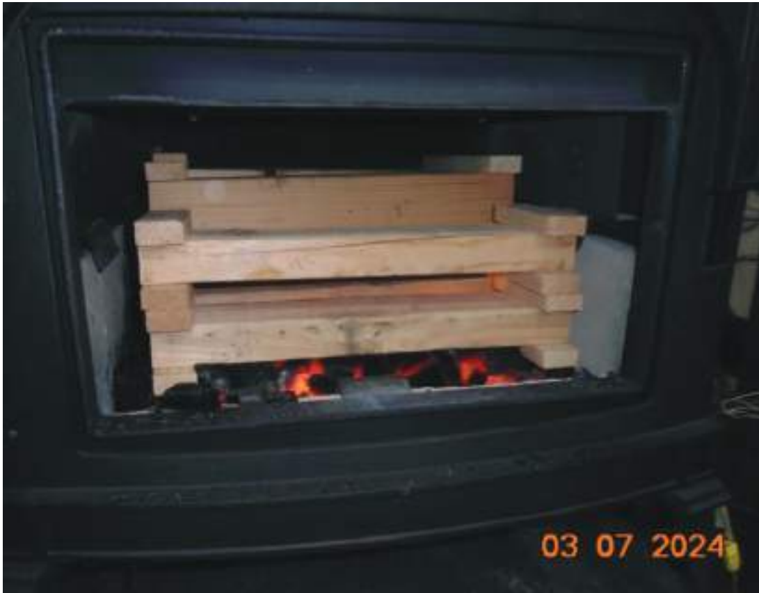
Figure 34 - Run 6 - Loaded Stove
