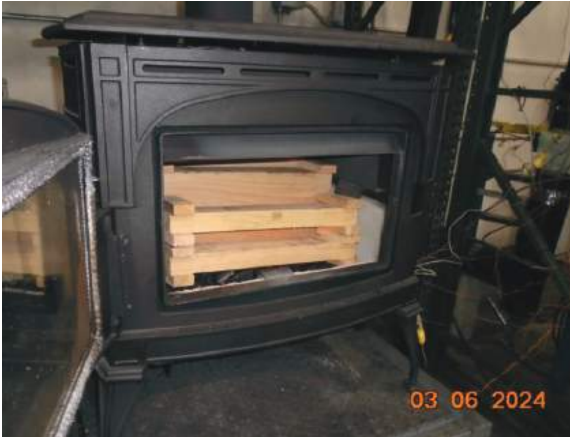
Figure 30 - Run 4 - Loaded Stove
