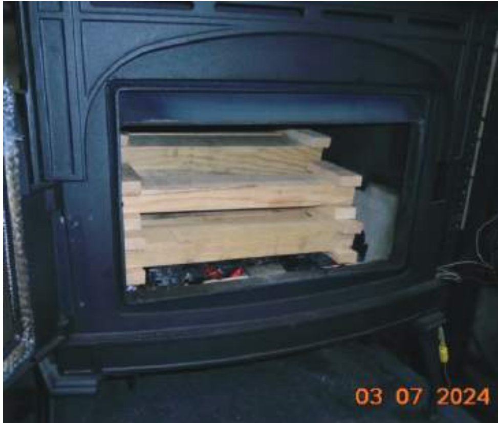
Figure 32 - Run 5 - Freshly Loaded Stove
