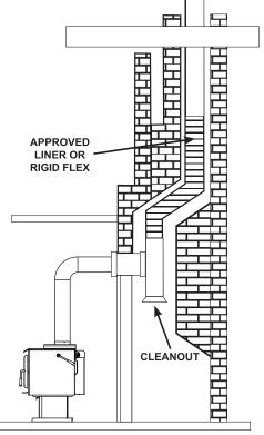
Typical Mason Chimney Installation Blaze King Recommend Installation
