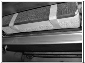
6. Before installing, align the combustor within the opening of the dome housing. Slowly push the combustor in at the top and apply even pressure to the left and right corners. This will allow for a better view of the bottom edge for the final fitting. **DO NOT FORCE THE COMBUSTOR INTO THE OPENING. TAKE YOUR TIME AND WORK IT INTO PLACE SLOWLY.**
