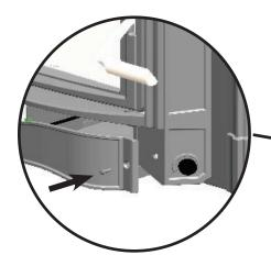
Note: If additional levelling is required, use only non-combustible material to fill any space under the appliance (ie. firebricks).
