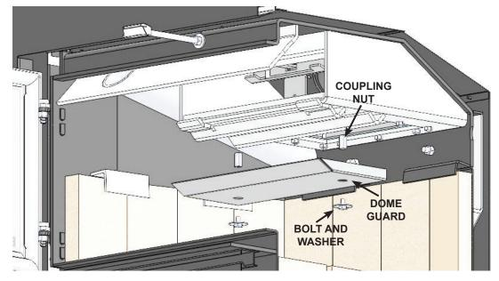
4. Remove the twelve remaining 1/4-20 nuts from the dome bottom. Lift the bypass door gasket retainer assembly upwards (enough to clear the threaded posts from the dome) and remove through the combustor opening. Once removed, ensure all debris is cleared from the inner surface of the dome. To reinstall the new bypass door gasket retainer, follow these steps in reverse order.
