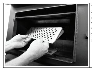
7. Once the combustor is fully reinserted into the opening of the dome housing, replace the flame shield. Note the flame shield sides are shaped like a triangle. The point of the triangle should face down to install correctly. Do not operate your appliance without the flame shield in place. The flame shield protects the face of the combustor against direct flame impingement and potential collisions when loading fuel.
