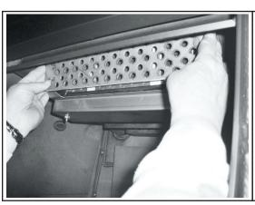
2. Once the flame shield is removed, you will have access to the combustor. The combustor can be made of different materials such as cordierite, mulite, or stainless steel. They are all the same with regard to removal and caution should be taken so as to not drop or damage the combustor. If your combustor has never been cleaned according the manufacturers directions, you may wish to clean the combustor before replacing it with a new combustor (please refer to the "COMBUSTOR CLEANING" section).
