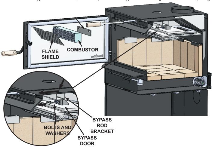
3. Remove the two 1/4-20 bolts and washers that hold the dome guard in place, be sure to support the dome guard during this process is it will come loose. Once the dome guard is removed, unthread the two 1/4-20 coupling nuts that spaced the dome guard from the dome bottom.
