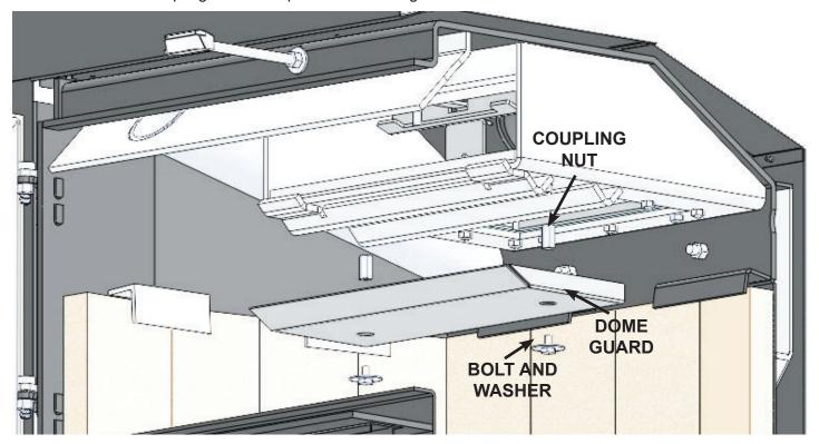
4. Remove the twelve remaining 1/4-20 nuts from the dome bottom. Lift the bypass door gasket retainer assembly upwards (enough to clear the threaded posts from the dome) and remove through the combustor opening. Once removed, ensure all debris is cleared from the inner surface of the dome. To reinstall the new bypass door gasket retainer, follow these steps in reverse order.
