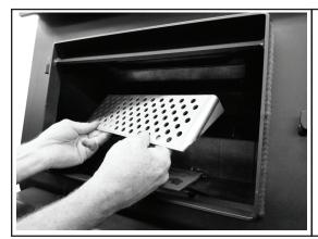
7. Once the combustor is fully reinserted into the opening of the dome housing, replace the flame shield. Note the flame shield sides are shaped like a triangle. The point of the triangle should face down to install correctly. Do not operate your appliance without the flame shield in place. The flame shield protects the face of the combustor against direct flame impingement and potential collisions when loading fuel.
