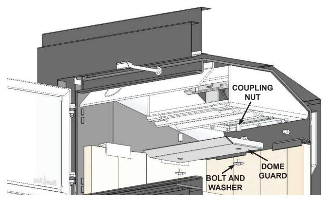
4. Remove the twelve remaining 1/4-20 nuts from the dome bottom. Lift the bypass door gasket retainer assembly upwards (enough to clear the threaded posts from the dome) and remove through the combustor opening. Once removed, ensure all debris is cleared from the inner surface of the dome. To reinstall the new bypass door gasket retainer, follow these steps in reverse order.
