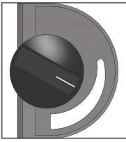
ROTATE COUNTER CLOCKWISE FOR REDUCED HEAT OUTPUT
