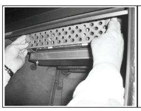
2. Once the flame shield is removed, you will have access to the combustor. The combustor can be made of different materials such as cordierite, mulite, or stainless steel. They are all the same with regard to removal and caution should be taken so as to not drop or damage the combustor. If your combustor has never been cleaned according the manufacturers directions, you may wish to clean the combustor before replacing it with a new combustor (please refer to the "COMBUSTOR CLEANING" section).
