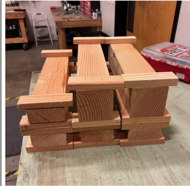
Test Fuel Front/Side View
